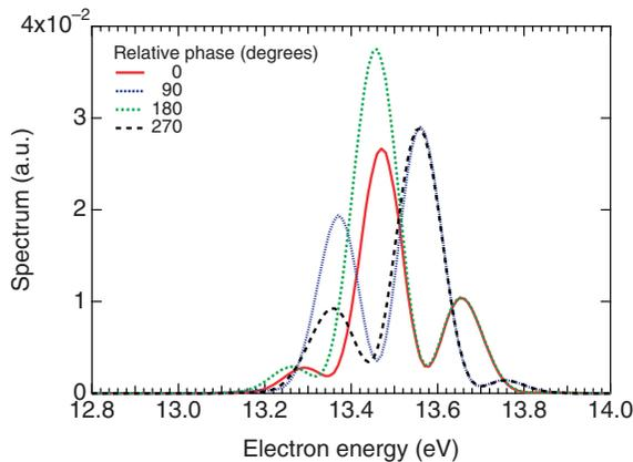
Figure 10. Two-photon ionization electron energy spectra by the double pulse with  $T=10$  fs and  $\hbar\omega=13.55$  eV with various relative phases  $\phi_{\text{rel}}$  at  $\tau=378$  fs. The relative phase is controlled by varying the delay between 1237 and 1238 optical cycles. (The color version of this figure is included in the online version of the journal.)
