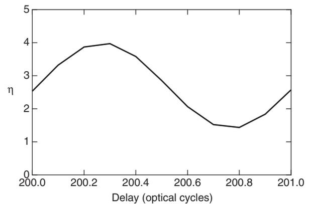
Figure 2. Oscillation of the ratio  $\eta$  of the ionization yield by double pulse to that by a single pulse as a function of the delay of the second pulse for the case of  $\hbar\omega = 13$  eV and  $T = 10$  fs.
