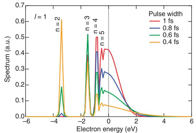
Figure 4. Energy spectrum of the  $p$ -state electron after the pulse with a photon energy of 13.65 eV and several different values of pulse width. (The color version of this figure is included in the online version of the journal.)
