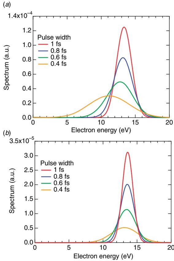
Figure 6. (a) Energy spectra of the electrons ejected through TPI by a pulse with a photon energy of 13.65 eV, a peak intensity of  $10^{13}$  W/cm<sup>2</sup>, and different values of pulse width. (b) Energy spectra of the electrons ejected through single photon ionization by a pulse with a photon energy of 27.3 eV, a peak intensity of  $10^{10}$  W/cm<sup>2</sup>, and different values of pulse width. (The color version of this figure is included in the online version of the journal.)
