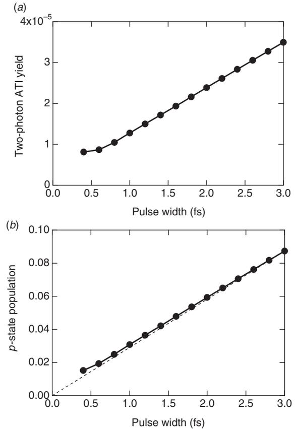
Figure 3. (a) TPI yield by a single pulse with a photon energy of 13.65 eV and a peak intensity of  $10^{13}$  W/cm<sup>2</sup> as a function of its pulse width. (b) The  $p$ -state population after the pulse as a function of pulse width under the same condition.
