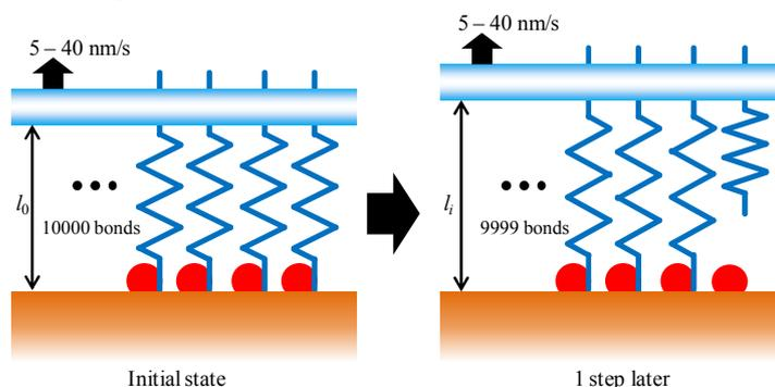
**Fig. 4** Schematic illustration of the calculation model for the experiment by Kim et al.<sup>(8)</sup>
