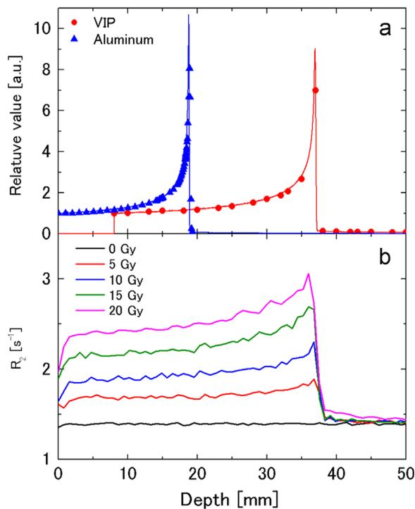
**Fig. 1.** Depth-dose distribution with 135-AMeV  $^{12}\text{C}^{6+}$ . (a) Distributions obtained with an ionization chamber using Al and VIP as range shifters. Symbols: measurements. Lines: PHITS calculation. (b)  $R_2$  distribution of VIP gels measured by MRI (Maeyama et al., 2014b).
