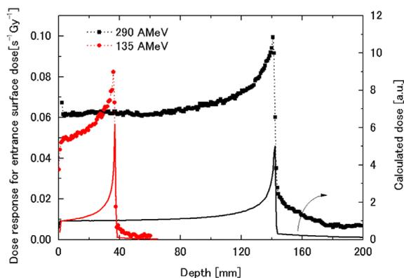
**Fig. 3.** Comparison between the dose response (symbols) and calculated dose distribution (solid lines) in the VIP gel with 135 and 290-AMeV  $^{12}\text{C}^{6+}$  (Maeyama et al., 2014b).
