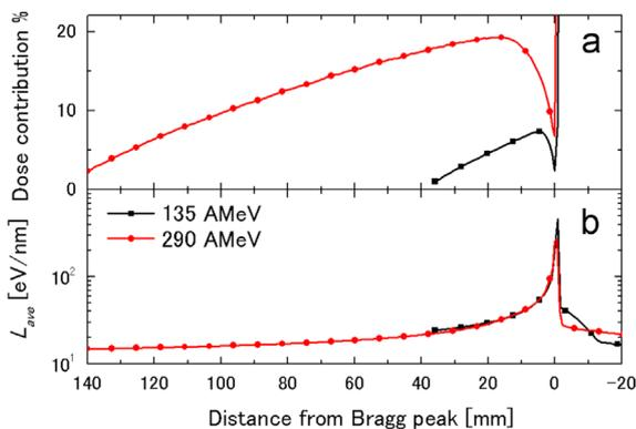
**Fig. 6.** (a) Relative contribution from secondary ions to dose and (b) dose-averaged LET for irradiation of 135-AMeV and 290-AMeV  $^{12}\text{C}^{6+}$  as a function of the distance from the Bragg peak.
