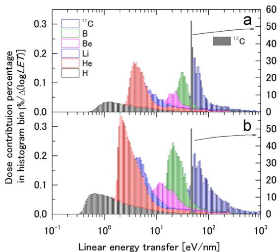
**Fig. 5.** LET distribution as a stacked histogram at the same dose-averaged LET (47 eV/nm) for 135 AMeV (a) and 290 AMeV (b). Open and solid bars correspond to secondary (left axis) and primary ions (right axis), respectively. Bin width  $\Delta(\log \text{LET})=0.054$ .
