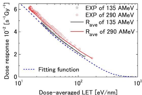
**Fig. 4.** Dose response of VIP gel for irradiation of 135 AMeV (squares) and 290 AMeV (circles) as a function of dose-averaged LET. The solid lines show dose-averaged response calculated from Eq. (2), and the dotted line shows the fitting curve from Eq. (3) as a function of mono-LET.
