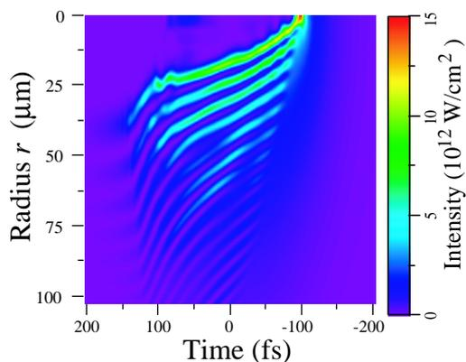
Fig. 1. Spatio-temporal intensity distribution of an initially gaussian pulse with an energy of  $135\ \mu\text{J}$  at  $z = 5000\ \mu\text{m}$ . Note that the pulse is symmetric around the beam axis  $r = 0$ .
