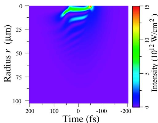
Fig. 3. Spatio-temporal intensity distribution of an initially gaussian pulse with an energy of  $15 \mu\text{J}$  at  $z = 7000 \mu\text{m}$ .
