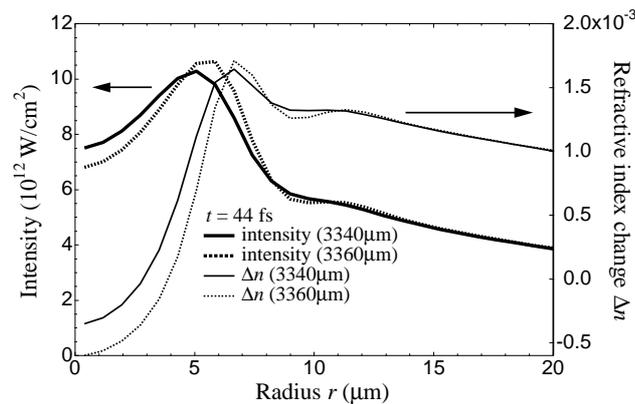
Fig. 2. Radial distribution of intensity (thick lines, left axis) and refractive index change  $\Delta n$  (thin lines, right axis) at  $t = 44$  fs. Solid lines are for the propagation distance  $z = 3340 \mu\text{m}$ , and dotted lines for  $z = 3360 \mu\text{m}$ .
