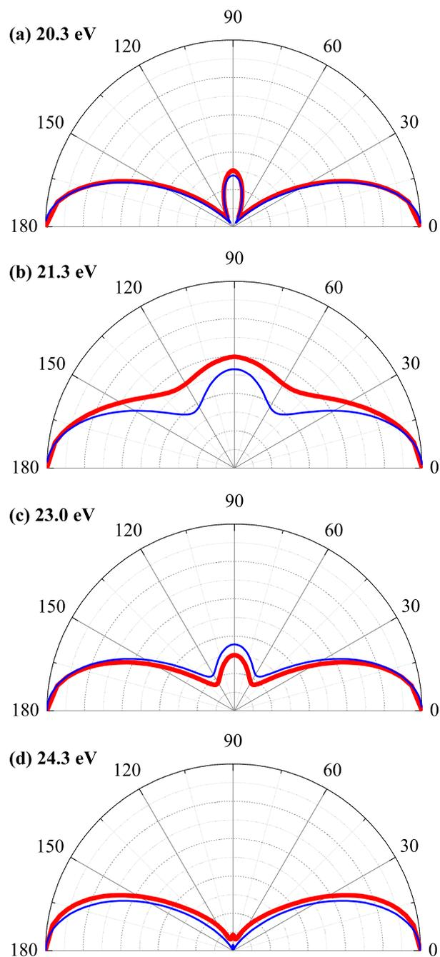
**Figure 2.** Measured (thick red lines) and calculated (thin blue lines) photoelectron angular distributions for two-photon ionization of helium. The experimental PADs are constructed from the  $\beta_l$  values extracted from the Abel inversion procedure.
