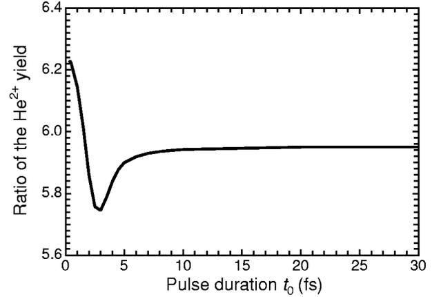
FIG. 5. The ratio of the  $\text{He}^{2+}$  yield at  $I_{\max} = 5 \times 10^{13} \text{ W/cm}^2$  to that at  $I_{\max} = 2 \times 10^{13} \text{ W/cm}^2$  as a function of pulse width  $t_0$  (FWHM) of a Gaussian pulse. The value expected for quadratic yield-intensity relation is 6.25.
