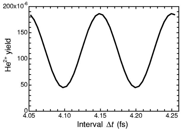
FIG. 9. He<sup>2+</sup> yield by a 27th harmonic double pulse as a function of the interval  $\Delta t$  between the two pulse peaks. Each pulse has a Gaussian temporal profile with a duration of 1 fs and a peak intensity of  $5 \times 10^{13}$  W/cm<sup>2</sup>. The first pulse peaks at  $t=2t_L$ .  $\phi_1=0$  and  $\phi_2=-\omega_X\Delta t$ .
