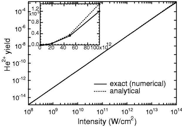
FIG. 1. Yield of He<sup>2+</sup> vs peak intensity of a Gaussian 27th harmonic pulse with a duration (FWHM) of 30 fs. The solid line denotes numerical results obtained by solving the TDSE, and the dotted line is calculated as  $\int_{-\infty}^{\infty} \sigma I(t)^2 dt$ . Inset: the same in a linear scale.
