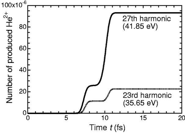
FIG. 7. Temporal evolution of the He<sup>2+</sup> population by two consecutive 27th harmonic pulses (solid line) and 23rd harmonic pulses (dotted line), respectively. The width (FWHM) of each pulse is 1 fs, the peak intensity is  $5 \times 10^{13}$  W/cm<sup>2</sup>, and the interval between the two pulse peaks is 3 fs.
