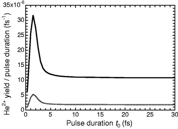
FIG. 4. The  $\text{He}^{2+}$  yield divided by the pulse duration (FWHM)  $t_0$  of a Gaussian 27th harmonic pulse with a peak intensity of  $5 \times 10^{13} \text{ W/cm}^2$  (solid line) and  $2 \times 10^{13} \text{ W/cm}^2$  (dotted line) as a function of  $t_0$ . Note that this quantity would be constant for the case of linear dependence of the yield on pulse duration.
