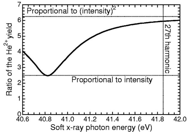
FIG. 3. The ratio of the yield He<sup>2+</sup> at  $I_{\max} = 5 \times 10^{13}$  W/cm<sup>2</sup> to that at  $I_{\max} = 2 \times 10^{13}$  W/cm<sup>2</sup> as a function of photon energy  $\hbar\omega_X$  of a Gaussian pulse with a duration of 30 fs. The upper dotted line indicates the value (6.25) expected for quadratic yield-intensity relation, and the lower (2.5) for linear relation.
