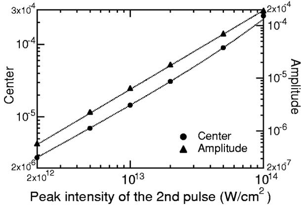
FIG. 10. The center (circle, left axis) and the amplitude (triangle, right axis) of the oscillation of the number of  $\text{He}^{2+}$  produced by the second pulse as a function of its peak intensity. Each pulse has a width of 1 fs, and the peak intensity of the first pulse is  $5 \times 10^{13} \text{ W/cm}^2$ . Dotted lines are the fitting curves obtained using Eq. (4.3).
